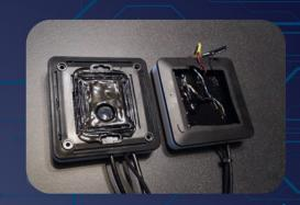
E3 Black Box records and saves driving condition information to replicate weather and road conditions, behavior the driver, behavior and dynamic changes of the car.
